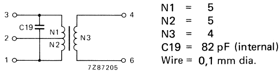
Fig. 13 Primary ratio detector coil (L3). TOKO sample no. 119 AN-7 P.
